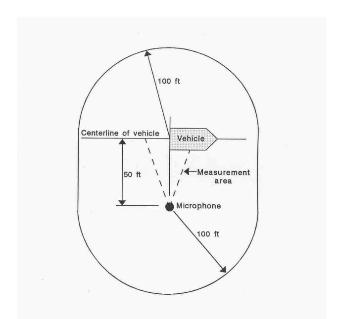
Figure 7.2-3. Test Site - configured for stationary tests.
